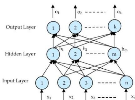
Fig 3. Basic block of Back-propagation neural networks
