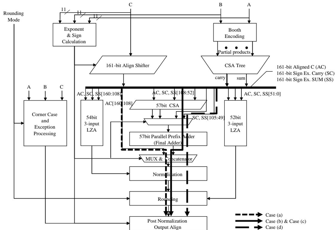
Fig. 1 Architecture of the proposed FMA unit according to the result of the sticky-bit generator and the round mode.
