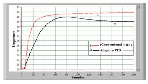
Figure 15. Comparison between adaptive PID and conventional PID controllers (setpoint equal to 30°C)
