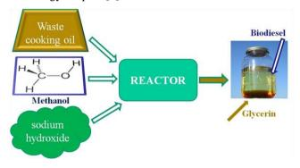
Figure 1. Schematics of biodiesel production from waste cooking oil.
