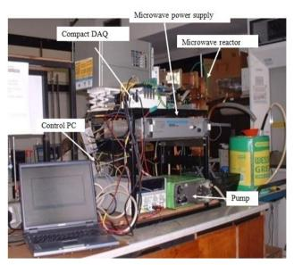
Figure 2. Developed biodiesel system.
