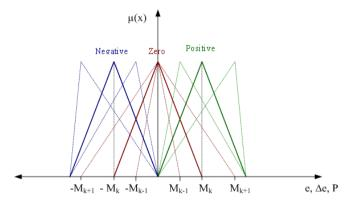
Figure 10. Triangular MFs modification according to the ILC law.
