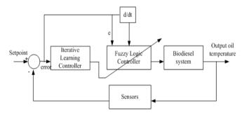
Figure 8. Self-learning Fuzzy Logic controller using ILC.
