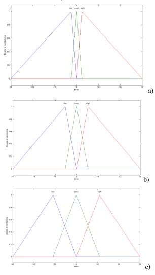
Figure 11. Modification steps of MFs for error in 300ml/min flow rate: (a) at inlet temperature, (b) at 30 °C setpoint, (c) at 35 °C.
