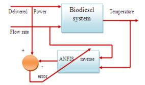
Figure 12. Block diagram for inverse control method.
