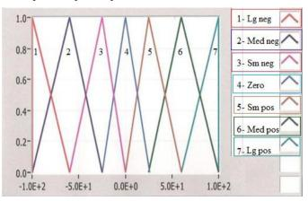
Figure 7. Membership functions of the output linguistic variables.
