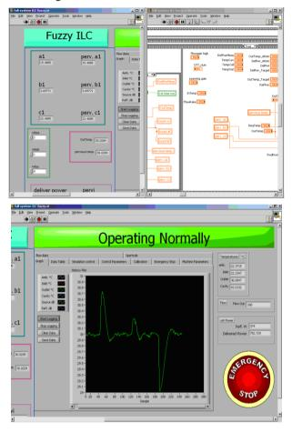
Figure 4. LabView control of the biodiesel reactor operation.
