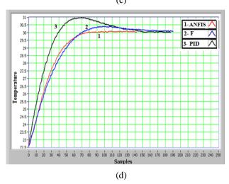
Figure 18. Controllers setpoint tracking comparison from inlet temperature,
