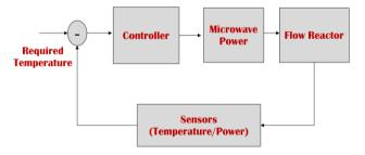
Figure 3.Block-diagram of the process, where microwave power supplied to flow reactor is regulated by a controller via temperature/power sensors of feedback loop.
