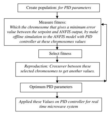
Figure 17. GA process in microwave biodiesel reactor
