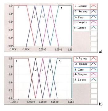
Figure 6. Fuzzy inputs membership functions (a) error, (b) change of error.
