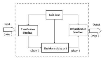
Figure 5. Basic block diagram for a fuzzy controller [3].
