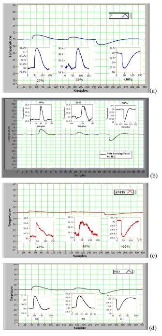
Figure 20. Disturbance rejections for the controllers: (a) Conventional fuzzy controller, (b) Self-learning using (ILC) controller, (c) ANFIS, (d). Adaptive PID controller.
