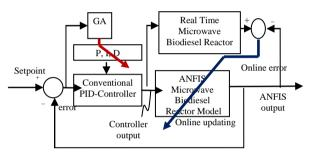
Figure 14. GA use as offline stage for tuning the PID parameters based on ANFIS mode
