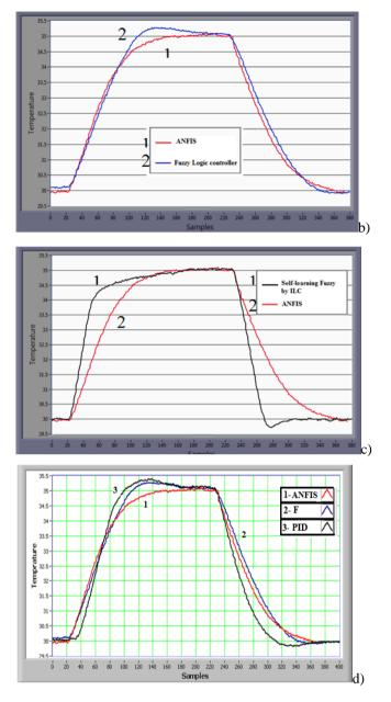
Figure 19. Controllers comparison on multiple sepoint tracking from nominal temperature value, (a) Self-learning using (ILC) controller and conventional fuzzy controller, (b) ANFIS and conventional fuzzy controller, (c) ANFIS and Self-learning using (ILC) controller, (d). ANFIS, conventiona FLC, and PID.
