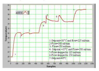
Figure 13. ANFIS controller output under different operation conditions.
