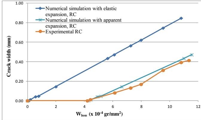
Figure 10. Relationship between corroded steel and crack width of RC beam
