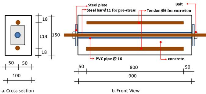
Figure 1. Specimen of RC and PC beam
