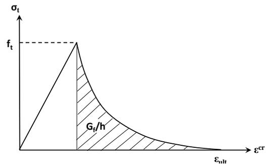
Figure 4. Constitutive model of concrete in tension
