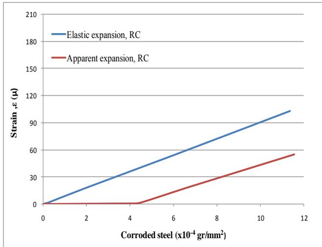
Figure 7. Corrosion expansion in RC member
