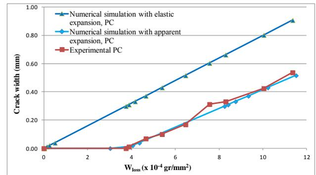
Figure 12. Relationship between corroded steel and crack width of PC beam
