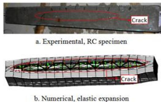
Figure 9. First crack on surface of RC beam
