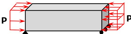
Figure 6. External compressive loads
