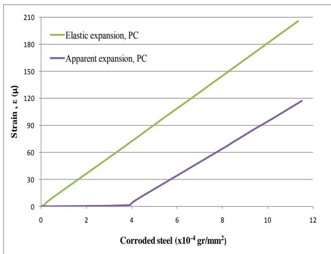
Figure 8. Corrosion expansion in PC member
