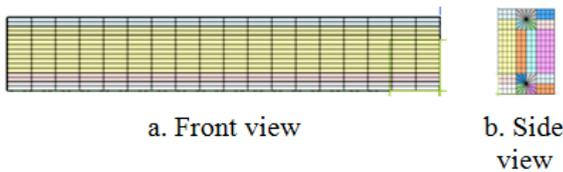
Figure 5. Meshing of specimen
