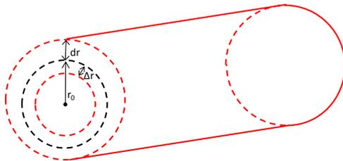
Figure 3. Corrosive expansion in cross section of steel bar
