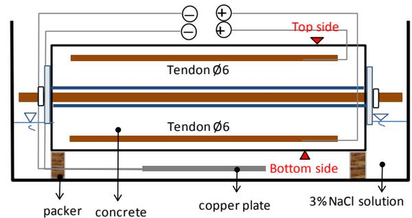
Figure 2. Schematic of corrosion test
