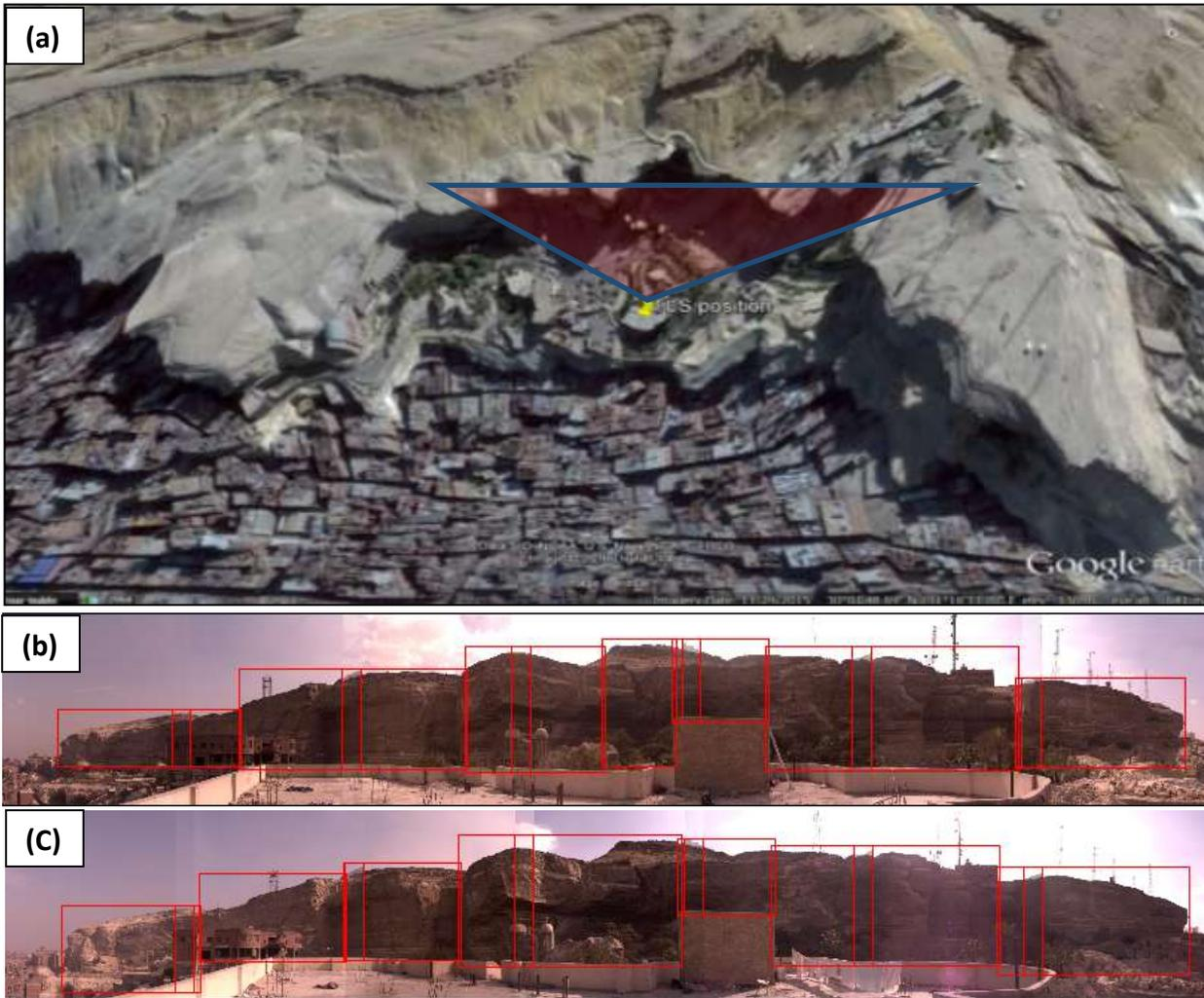
Figure 2. (a) Google earth satellite 3D image of El Mokattam plateau showing the position of the TLS. (b& c) The scan areas in 2012 and 2013 respectively (the red boxes show the different scan tasks)
