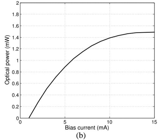
Fig. 4. Static characteristic of the studied VCSEL - (a) Simulated curves - (b) Measured Finisar Photonics curve [10].
